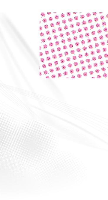
The picture shows a magenta halftone, simulated on a proofer. The basis of the halftone is the light magenta ink of the proofer, but the normal magenta ink is also used to make it darker (see the darker magenta pixels). Light cyan and yellow contamination pixels are also visible, making it less saturated, and obtaining the right color. The frequency of this screen is 170 lpi, resampled from 2400 dpi to 1440 dpi.
