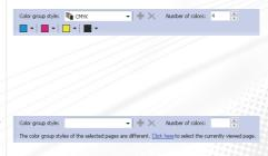
New *color group styles* can be created and saved if the same color combinations are being used regularly. For example, if two colors (e.g. blue and orange) are often printed but are printed as cyan and magenta. Define the two colors used, making a *color group* of these two colors, and then save it as *Blue and orange* color group style. It is then possible to change any subsequent jobs by one click into *Blue and orange*.
